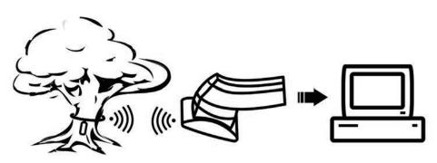
RFID Tag (with string, ring, label) **RFID Reader**
